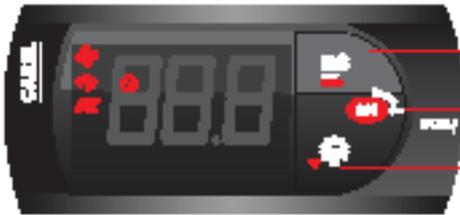
Temperature is increased by pressing this button after setting the device temperature. It is activated when the set button is pressed for 2-3 seconds.
